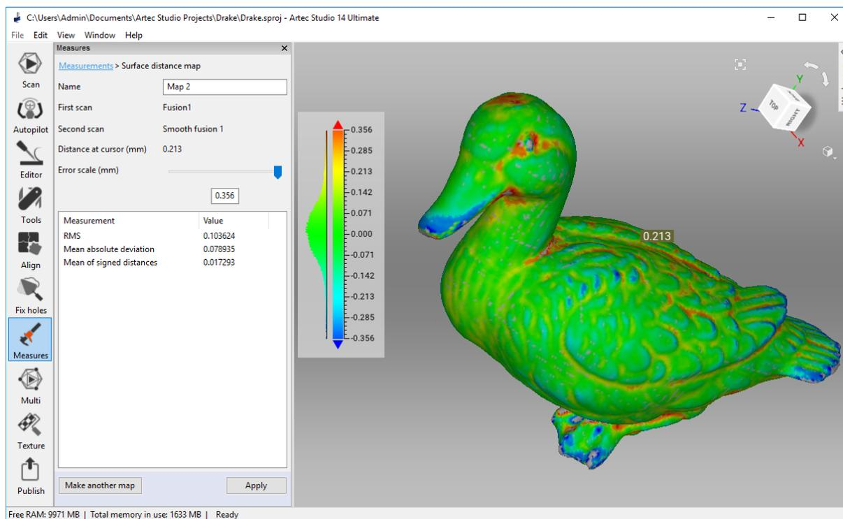
Figure 117: Surface-distance map calculated for two models.
