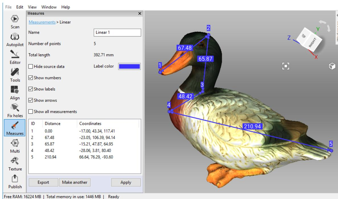
Figure 112: Linear measurement.
