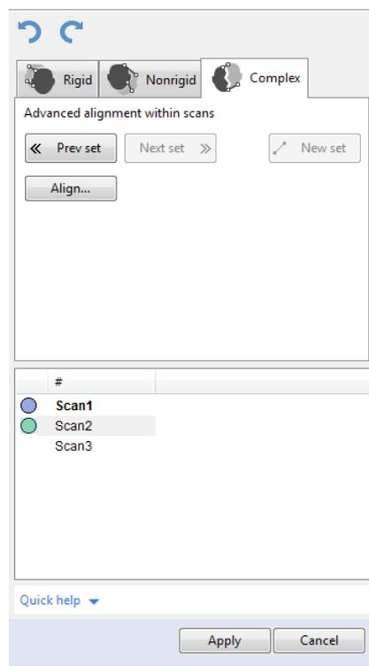
Figure 72: Align panel: Complex tab.
