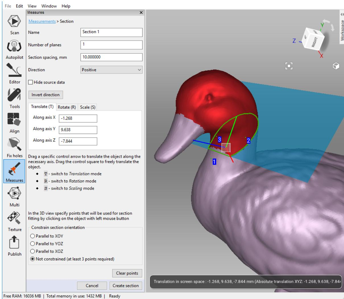
Figure 114: Orienting new section in *Translate* mode.
