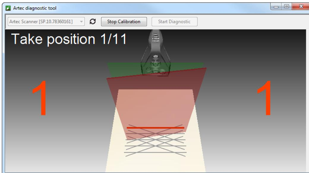
Figure 138: Moving calibration rig to position number 1.
