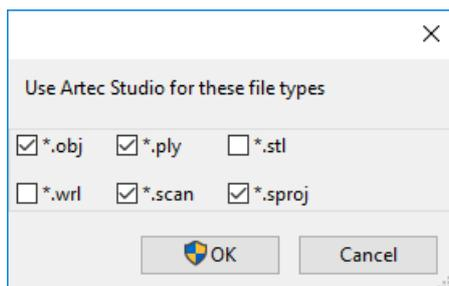
Figure 120: Making Artec Studio the default application for various file types.
