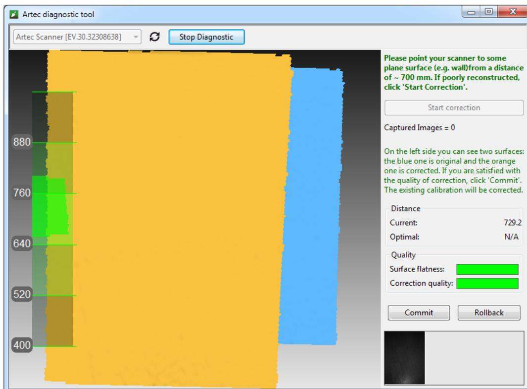
Figure 129: Artec EVA correction results.
