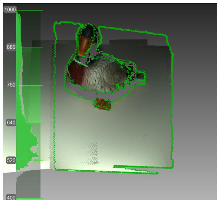
Figure 29: Texture tracking renders color object (scanner's current field of view outlined in green).
