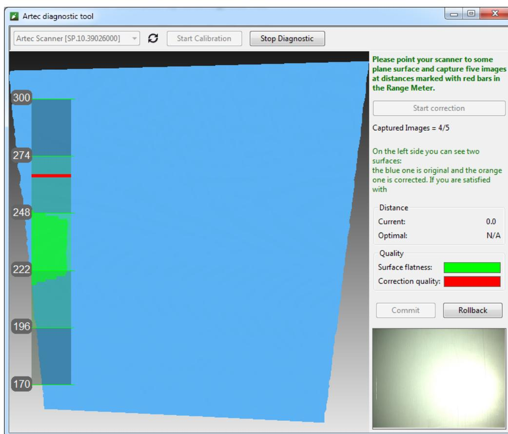
Figure 130: Artec Spider correction process.
