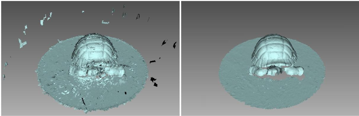
Figure 58: *Outlier removal*: before and after.
