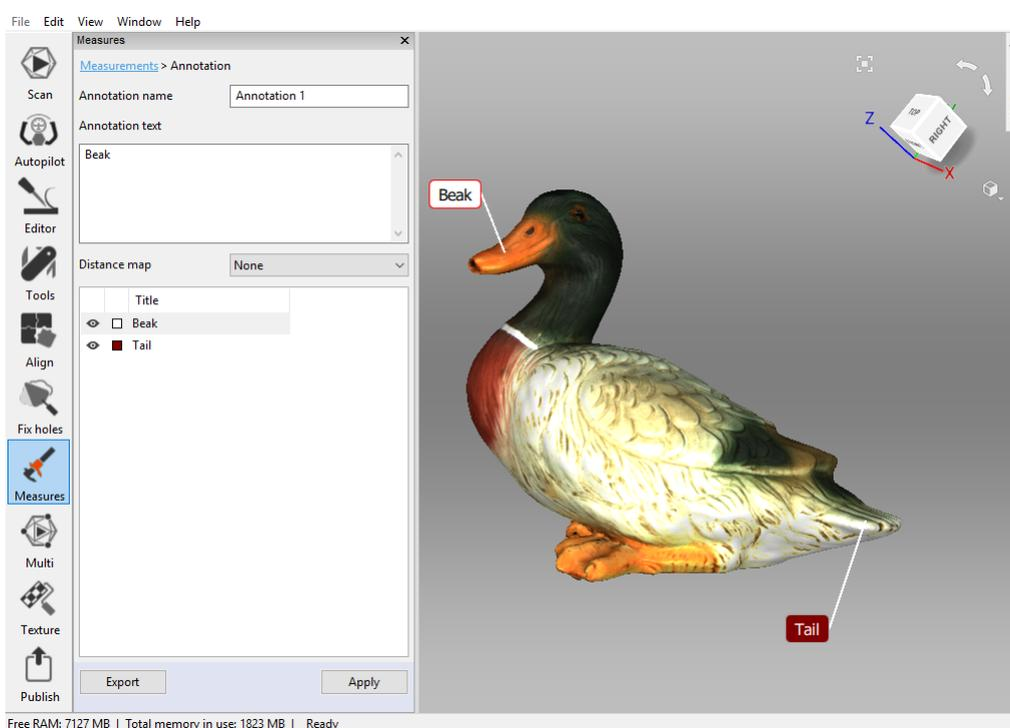
Figure 118: Annotation of a model layered with a surface-distance map.
