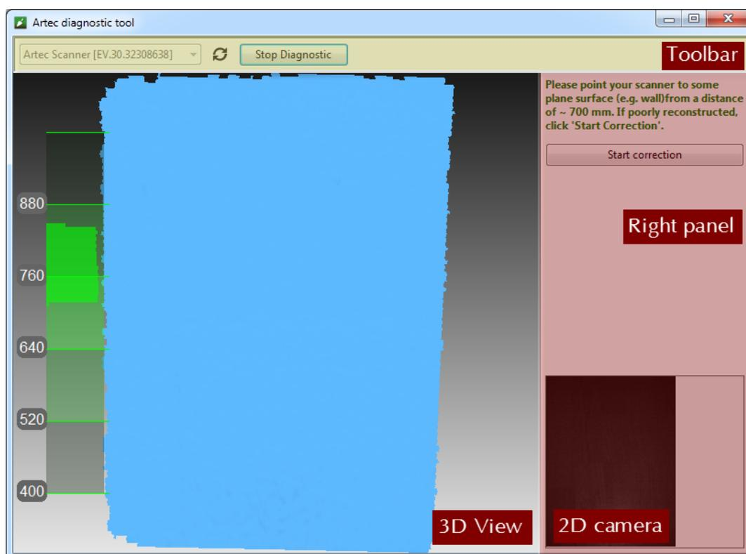
Figure 128: Diagnostic Tool window.
