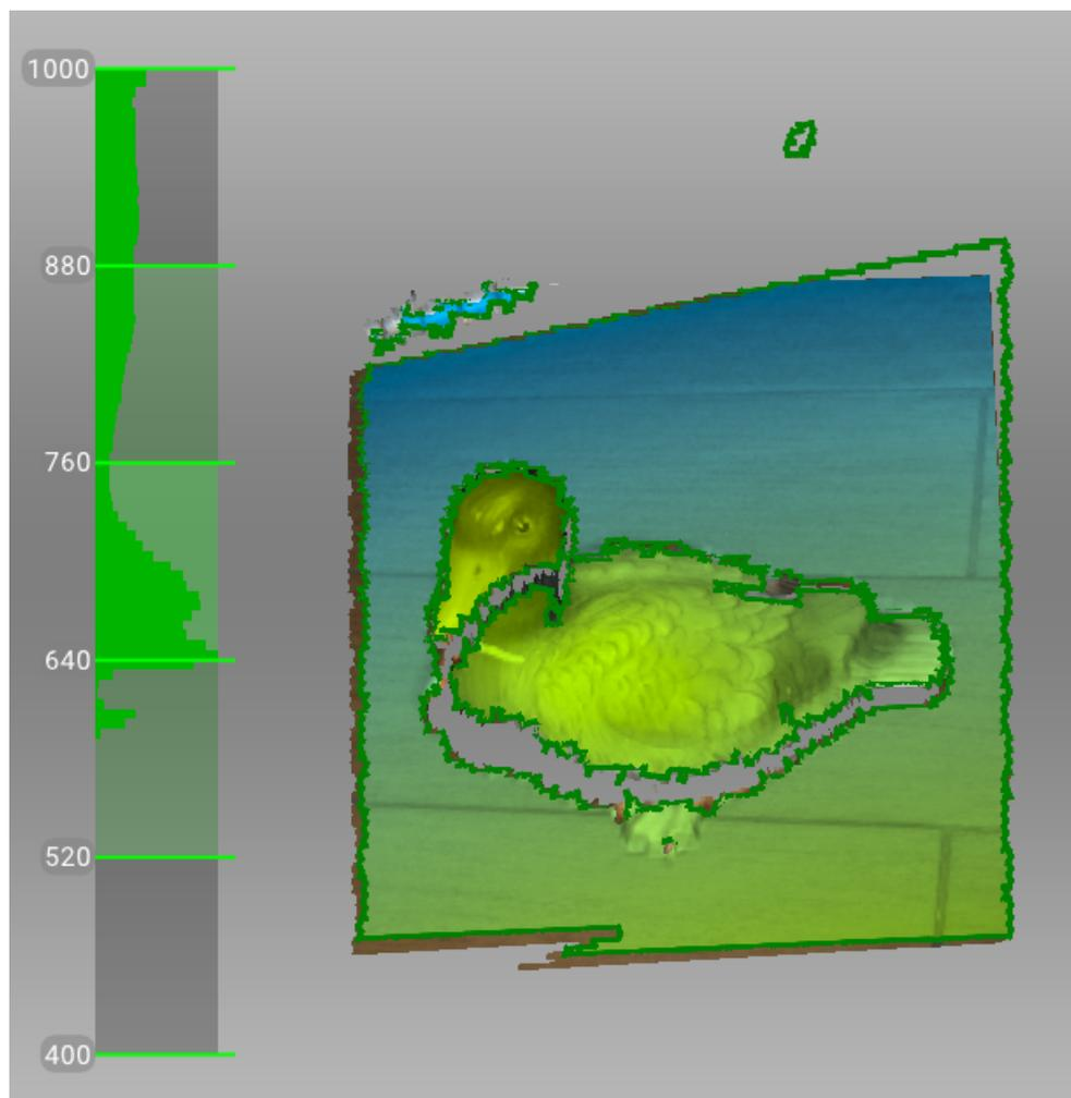
Figure 28: Distance meter and distance color showing surfaces that fall within the optimal range for Artec Spider.
