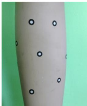
Figure 35: Non-coded targets placed on an object.
