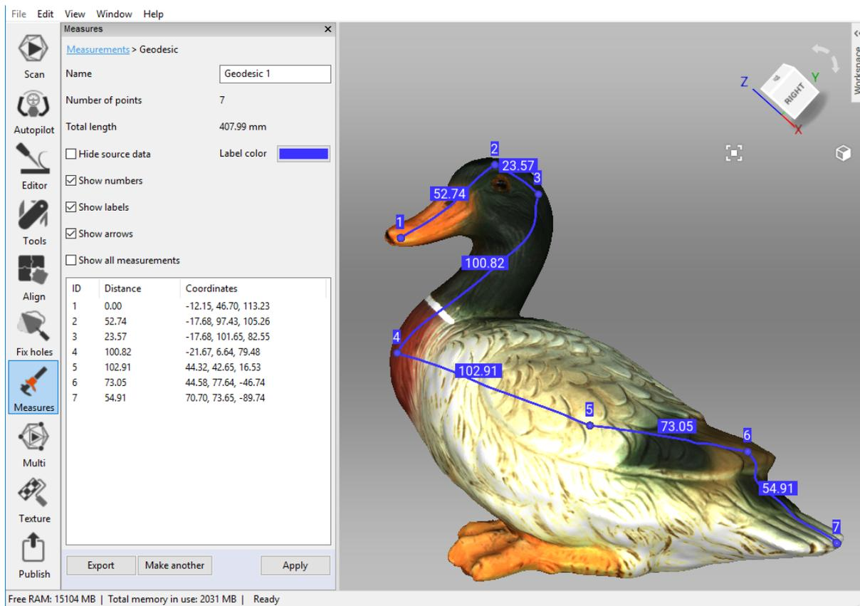
Figure 113: Geodesic-distance measurement.
