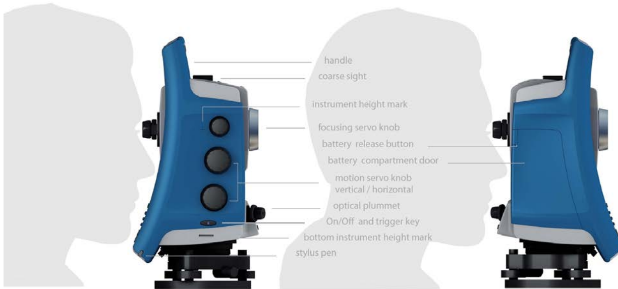
Figure 1: FOCUS 35 design and ergonomic features
