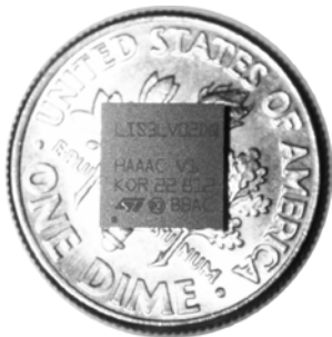
Figure 8: Size comparison of an MEMS acceleration sensor
