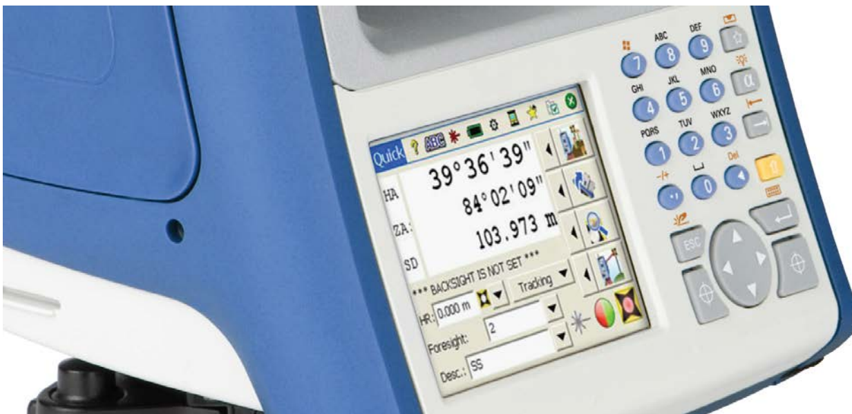
Figure 15: FOCUS 35 control unit with Survey Pro application software
