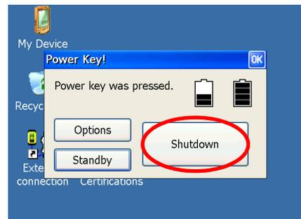
***Note** – Executing Shut down ends the application program and the data that are not stored in the program will be lost.*
