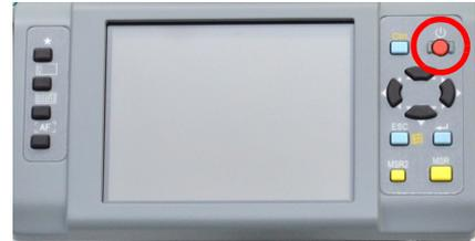
***Note** – Check the batteries are correctly inserted into the slot if the application program doesn't start up even after pressing [power].*
