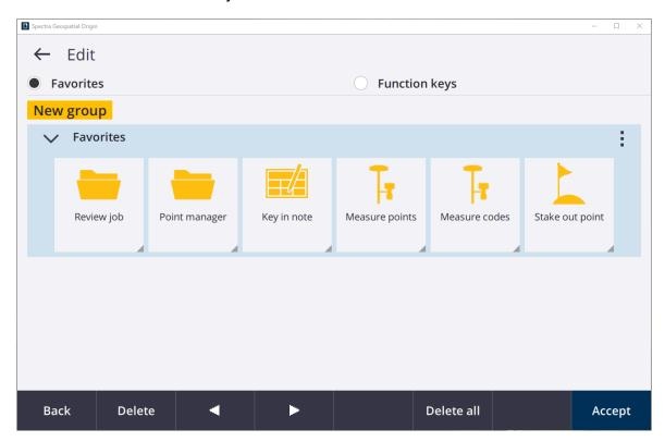
3. To rearrange the icons, use the two arrows at the bottom of the screen.
