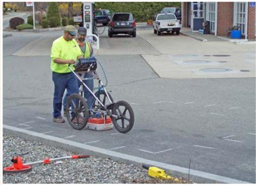
Picture shows complementary GPR system, UtilityScan™
