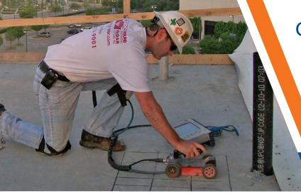
Complete GPR System for Concrete Inspection and Analysis
