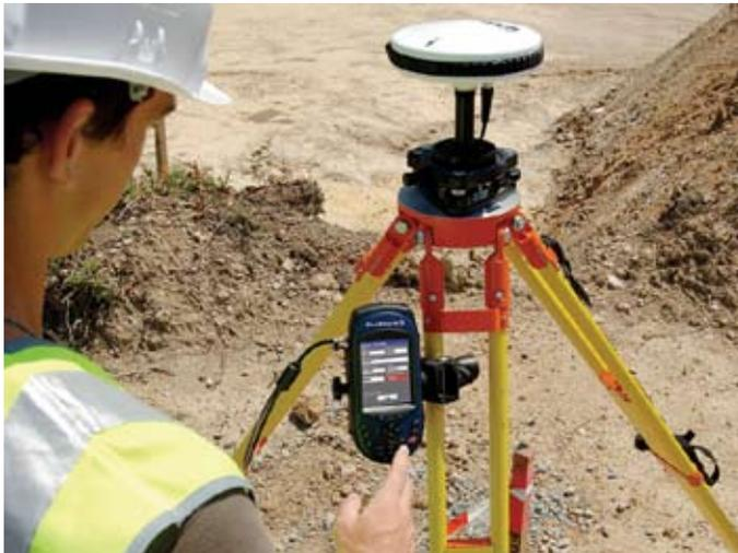
Locating and surveying hard-to-find points is a snap with the navigation and data collection capabilities of ProMark3. After navigating to a point using the unit's base map, transitioning to survey mode requires only a single keystroke.
