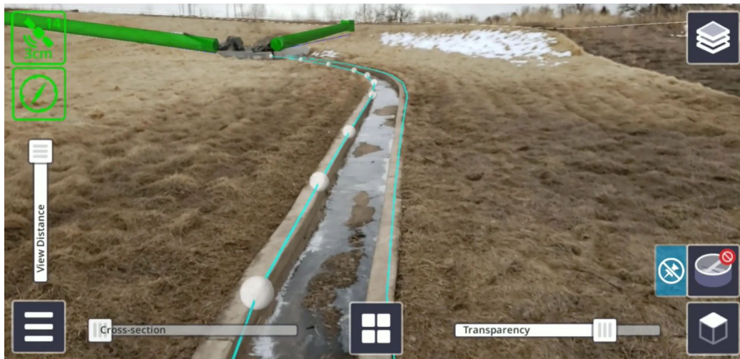
Figure 4 - TBC processed survey data and published georeferenced data to Trimble SiteVision
