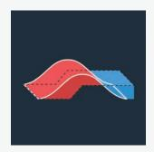
Compare volumes between two surfaces. This could be survey to survey, in order to see changes and progress over time, or measure against a design surface to see how far you have left to go.
