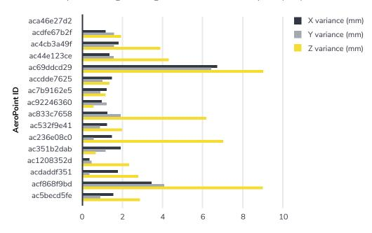
For our first flight, we calculated the variances in each dimension for all the AeroPoints used in this survey. They reported internally consistent numbers as processed using the known-point method.
