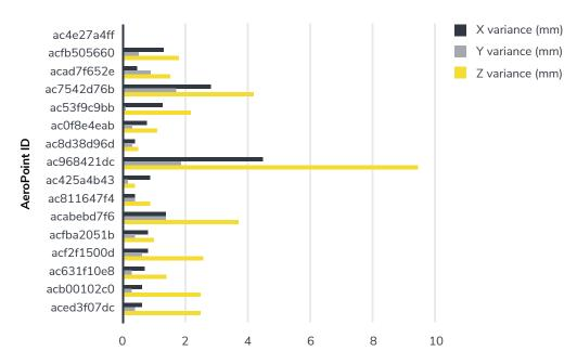
In the second flight, we again calculated AeroPoint positional accuracy. All AeroPoints again reported internally consistent numbers as processed using the known-point method, with no individual point getting less than 1cm accuracy, and most falling well better than that value in the height dimension.
