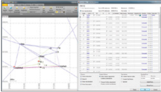
Adjust leveling data and integrate into network adjustments
