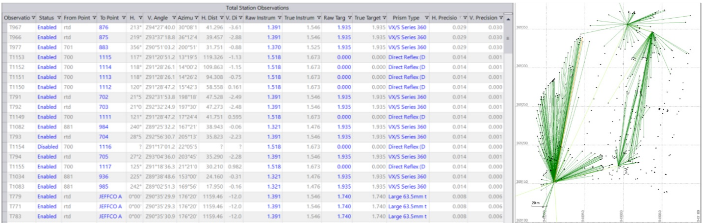
Figure 15 – Total station observations (green) and Optical Spreadsheet in TBC – Notice the “from point” and “to point” columns
