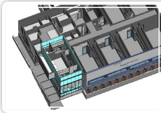
3DIS used EdgeWise Building to convert laser-scanned data into a usable format for 3D modeling
