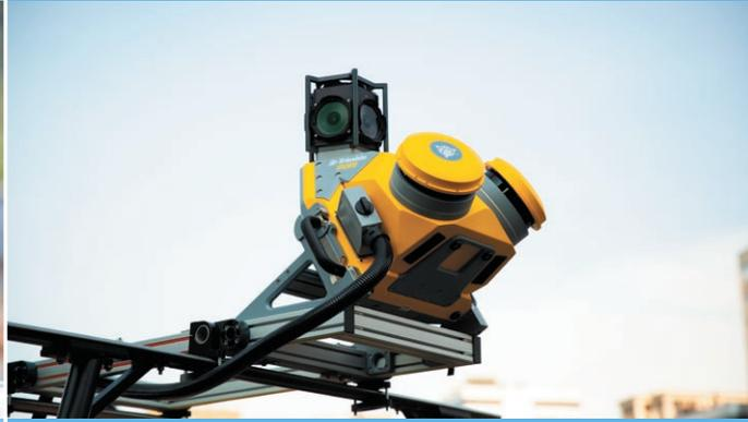
The Trimble MX50 is a practical field-to-finish mobile mapping solution for asset management, mapping, and road maintenance.
