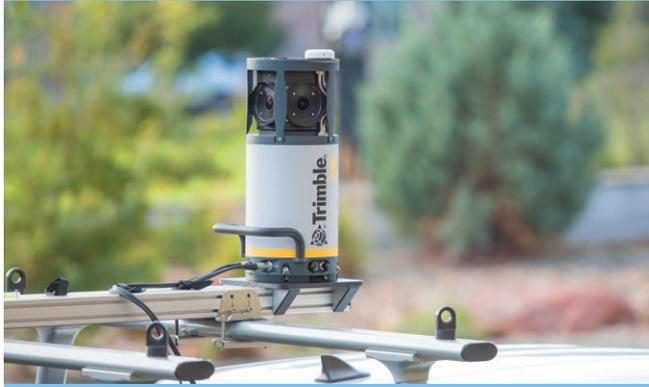
The Trimble® MX7 is a vehicle-mounted imaging system enabling fast and productive capture of road, infrastructure, and city environmental data. The system combines a 360° spherical camera with an integrated Trimble GNSS/ Inertial positioning system giving you the capability to position objects photogrammetrically from an accurate vehicle trajectory.
