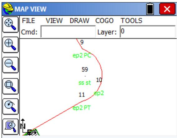
To remove the bulge in the arc and make it tangent, add code "AFIT" to point 10. If Line Details are clicked on within Configuration, the moment you add the text (click 10 directly in map screen and edit it), the line will redraw as shown below. In the field, if you add AFIT ahead of time, anticipating a bulging arc, it will draw correctly in the field.
