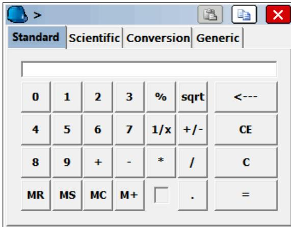
This leads immediately to the Calculator dialog, with its four tabs, or options, many with sub-options. Using the Standard tab, we can enter  $0.12+0.15+0.33+0.25$  and then "=". Then select the Copy button, which places the value in the banner line at the very top of the screen. Then choose Paste to paste the value back into the Vertical Offset dialog edit box. Change the sign to "-" for negative, as needed. Calculations can also be done directly from the edit box within the Vertical
