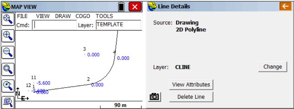
You have the option to delete the line or change its layer or View Attributes (if any). If the polyline (a line with 2 or more vertices) has different elevations on some of the vertices, then it is designated a "3D Polyline". A more advanced Line Details is provided when using Feature Codes within the Store Points command, allowing extension of lines and new lines from vertices on the polyline. The advanced Line Details is discussed under File, Feature Code List.
