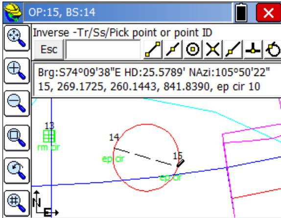
Third, if 3 points are entered as in 9 code CIR, then 10 code, then 11 code CIR, the third point defines a unique circle without user entry of the radius. This is shown in the above graphic. The code used must be a linework code (like EP for edge-of-pavement), not a point code, for the circle to be drawn.
