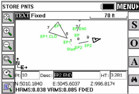
The above figure displays the next EP code EP2 stored using GNSS Simulation. When ended with a END or CLO description after EP2 SurvCE will prompt for EP GIS data to attach to the polyline as defined above.
