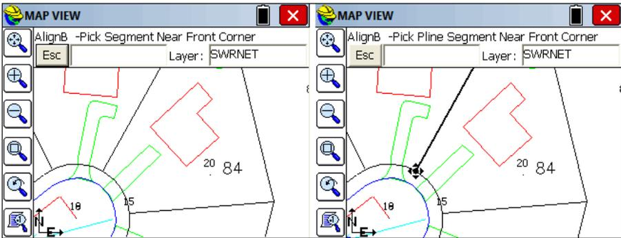
**Pick Pline (Building) Segment Near Front, Lot Side:** Pick the same lower left building corner as shown above, but along the side facing the adjoining lot line. This leads to the graphic below. The correct side line is highlighted.
