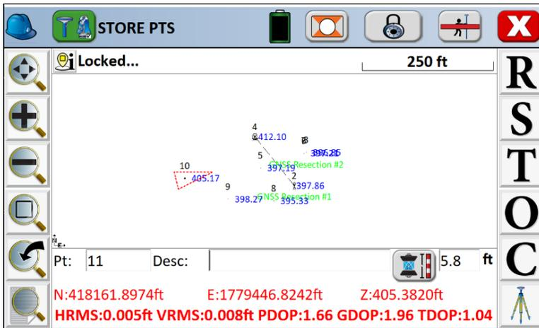
*Shown in the image above, the robotic total station is the active instrument, but is in a locked state (the E.D.M. is not firing). Since no position is available from the active instrument, and backup tracking is enabled, SurvCE is displaying the backup position of the GPS in red.*
