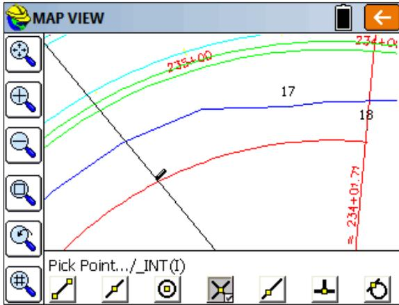
The road section from 234+00 to 236+00 is in a spiral curve and the goal is to intersect the right-of-way of the road, which is at a 50' offset from the centerline, with an original property line running NW to SE. Rather than use complicated coordinate geometry, the Map screen can be used to select Draw, Offset and create a 50' offset line of the road, shown above. Then within Stake Points, where point 17 is the occupied point and 18 is the backsight point, the point to stake can be
