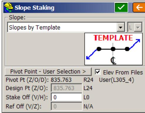
**Define Slope by Next Section Point:** This option allows you to select the edge of the road and use the proposed design catch point for auto-determining the slope rate.
