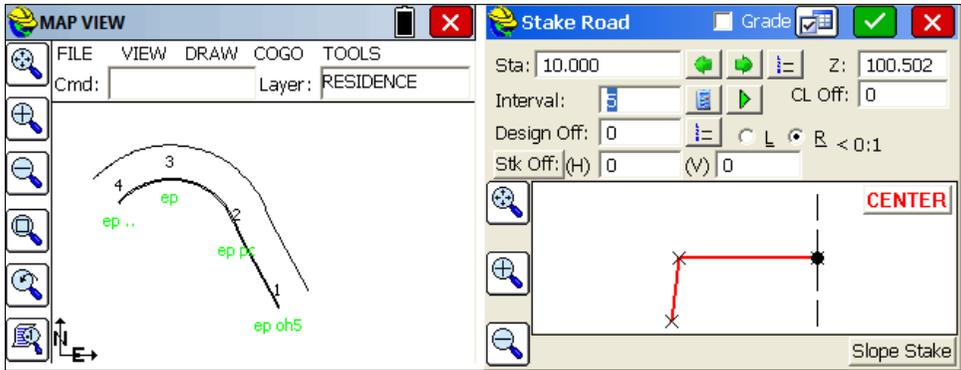
Using the "Interval" method (normal method), vertical offsets can be by elevation difference (default), or by slope percent or ratio. The default "Continuous" option keeps the offset 3D Polyline as a single entity. If you do the "Segment" option approach, only the segments of the 3D polyline will offset (leaving gaps), and you have the option to create Point IDs on the offset vertices.
