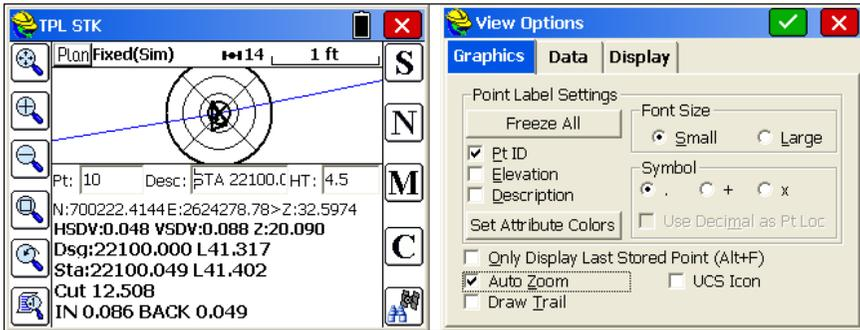
The "Story Stake" information would appear as shown below (Progressive and Total options). By staking Section ID "Ditch", there are 2 Ditch ID points to the left and 2 shoulder and 1 Center point to the right, up to the selected centerline.
