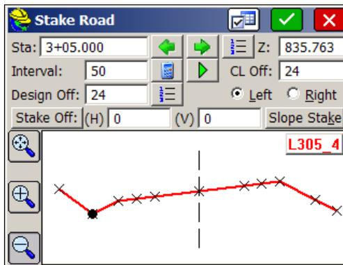
If you click Slope Stake, you can stake by the template slope for the ditch shown on the left side, or you can enter a user-defined slope to override what is in the template.
