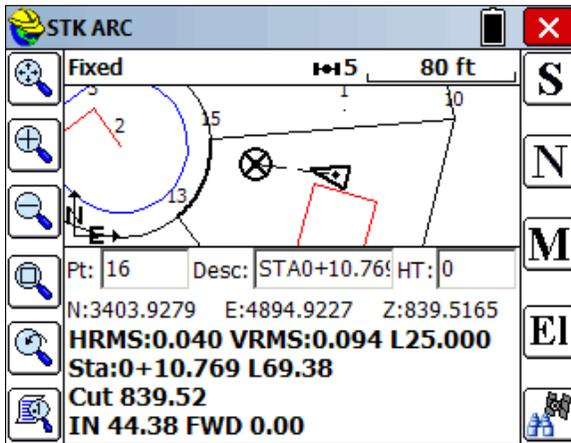
The above example might be useful for setting stakes at a 25' building setback from the right-of-way line. For GPS, information is provided "real-time". As you move, you see the instructions to contact the nearest point on the arc (or offset to the arc). For total stations, you are first instructed to measure to the nearest point on the arc (or arc offset) from the instrument setup. Then after you take any shot, the instruction refers to that measurement.
