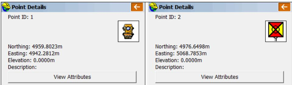
If you have assigned attributes to the points (e.g. Description Pole, Type-Metal, Wires-4, etc.) by use of the Feature Code capabilities, these attributes can be reviewed. The Point Details option works both within the MAP screen (when you are not being prompted for entering points or selecting objects) and in all graphic screens within the Menu options. It is not as transparent and available as the dynamic pan option, but nearly so.
