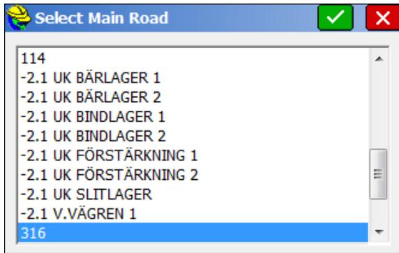
You then select any road to stake out, such as "316" in this example. Within the selected road, you can pick any surface (much like in the Cross-section method) and any point on the surface. If available, the description of the selected surface point is shown:
