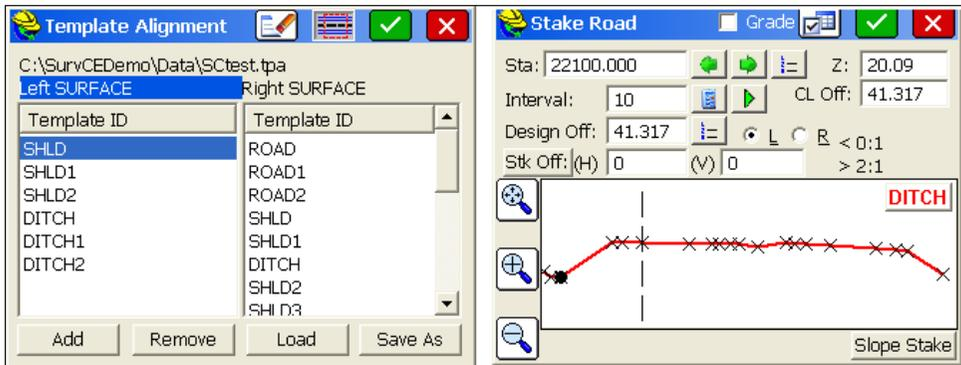
Note that when picking the first ditch point left side, that the layer is Ditch, and the next two are layered Ditch1 and Ditch2. Above the select Ditch point to the right is the third shoulder point on the left side, with SHLD2 as the ID. The next step is simply to click OK (green check) and start the normal stakeout process. Note also that you can Slope Stake (typically from the outer ditch point on the trapezoidal ditch, Ditch1 in this case).
