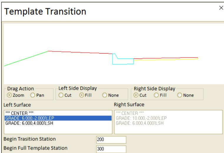
Note that at station 300, the full EP position is at Design Offset 6, based on the DEMO template transition file (DEMO.TPT). At station 250, the EP lane would be 8 units wide, halfway between
