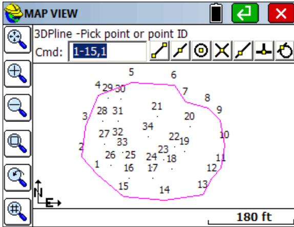
Finally, if you are doing a stockpile and make the effort to put this outer perimeter in the “Perimeter” layer, then you can select the “Stockpile” option within Volume, define the final surface appropriately, and click OK. You don't need any other definition for the original surface. This is because the Perimeter layer will define both the inclusion perimeter and the original surface in this case.
