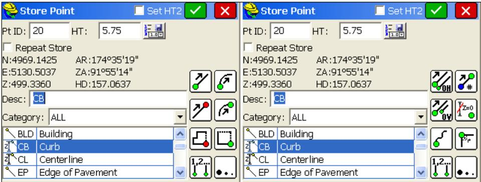
On the first page, these codes going from top to bottom, starting at the left, represent start line, end line, close line, select active line (when multiple lines are being drawn with the same code), start curve, end curve, rectangle, and "more". When you pick more, the options are offset horizontal, offset vertical, smooth curve, select active line, join to point ID, no elevation, jog and more (return to first set of icons).
