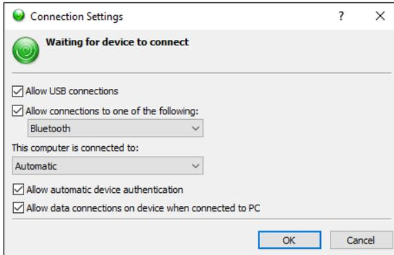
Be sure that you have selected the appropriate COM port or USB options. Upon connection of the mobile device (Surveyor 2 or other Windows Mobile Device), the program will recognize and begin the connection process. Sometimes however, this does not automatically happen and a disconnect / reconnect procedure may be needed. To ensure the mobile device is connected and recognized by the PC, a user may need to investigate the connection (Device Manager – COM Ports).
