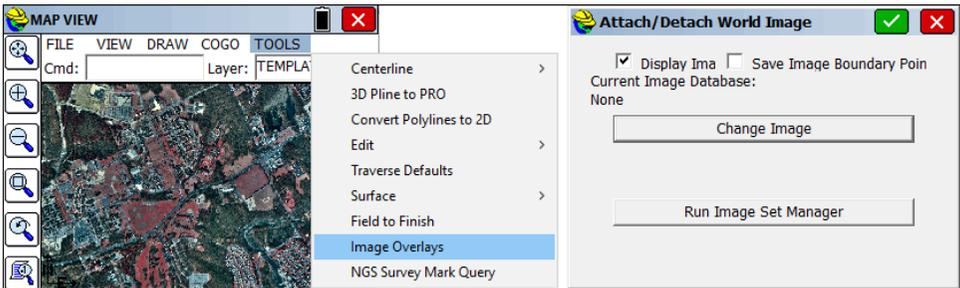
Images that do not have any georeferenced information built into them (or available in a separate jpw or tfw file) must be calibrated within Carlson X-Port, the office software companion to SurvCE, using the Image Manager. GeoPDF format is supported.
