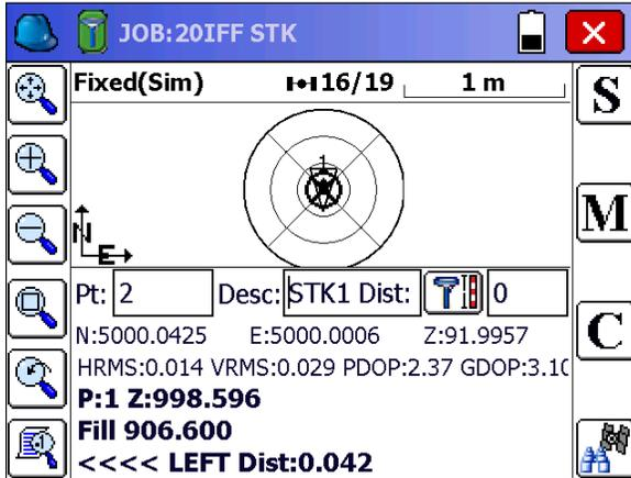
The screenshot shows a software interface for a stakeout. At the top, it says 'JOB:20IFF STK'. Below that, there's a status bar with 'Fixed(Sim)', '16/19', and '1 m'. A central bullseye target is visible. On the left, there are navigation icons. On the right, there are function buttons labeled 'S', 'M', 'C', and a printer icon. The main data area contains the following information:
