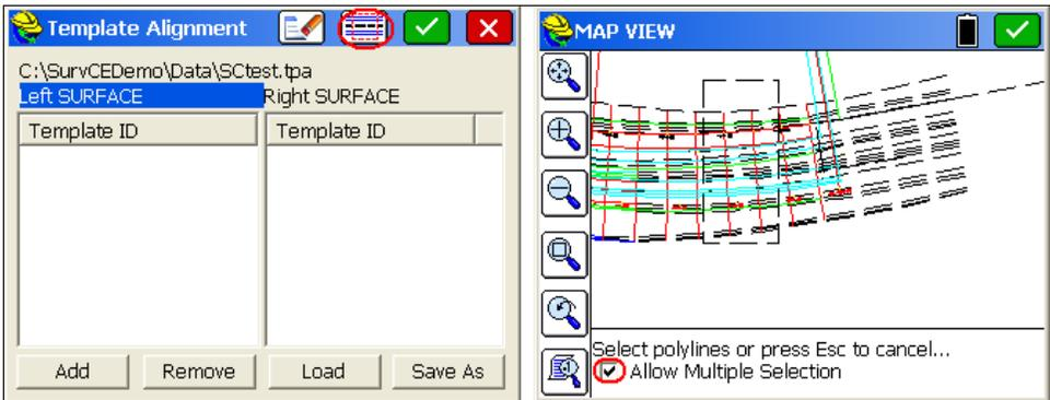
If there is previous data in the 2-column screen, use the Eraser Icon to delete all the data. Then rather than pick one polyline at a time, use the window/crossing selection icon circled in red above left. This leads immediately to a map screen as shown above right. In the lower portion of the dialog, click on "Allow Multiple Selection". Then do any combination of individual picks or window/crossing selections (lower left to upper right or lower right to upper left). A typical
