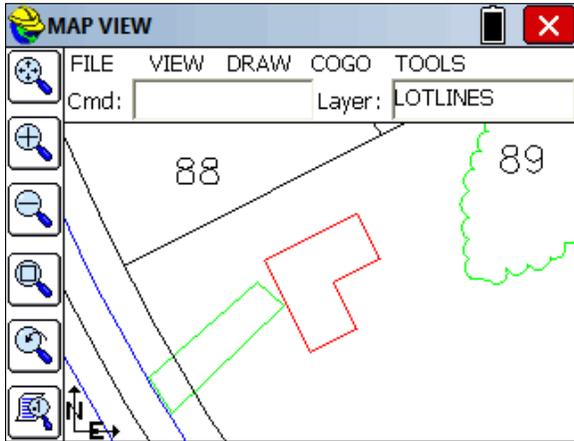
The **Scale** command operates much like the others by first requesting a base point for scaling, and then a scale factor: R for Ref is similar to rotate, where you specify the segment on the object that you are referencing and then the segment on another object you wish to match, for scaling.
