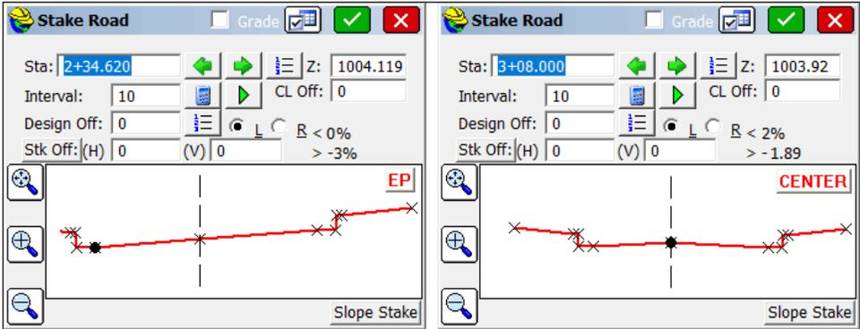
Clicking OK on station 234.62 above would lead to the following stakeout screen, as seen in Plan View (default) and Section View (click Plan/Section in upper left of screen to switch between views). The button shows current view status.
