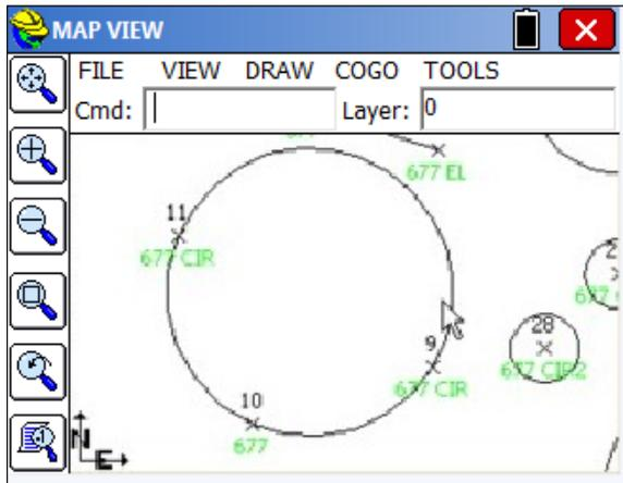
Secondly, if 2 points are used, then the radius becomes the mid-point of the 2 points and a circle will be drawn through both points with the entered radius:
