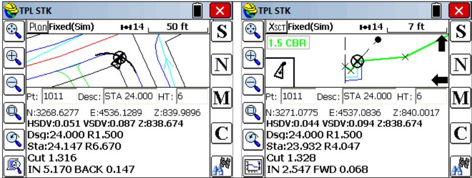
The process can be repeated for the cul-de-sac. Here we will stake out both the stone subgrade outside point and then we will slope stake the catch at a station approximately 1/4 of the distance around the cul-de-sac:
