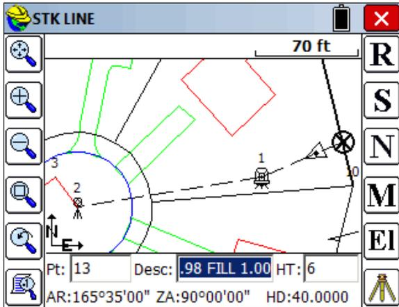
**Total Stations/GPS, Perpendicular to Line:** When configured for the Perpendicular to Line method, the program will show the direction and distance to move to find the nearest point on the line to the measured point. The instruction received (In/Out versus North/South or Azimuth/Distance) will depend on the setting within Configure Reading.
