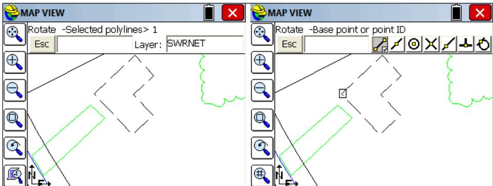
First you select the polylines to rotate. Press Enter when there are no more selections. Then choose your Base Point for rotation. Here, we use the Endpoint snap and select the corner of the building shown.
