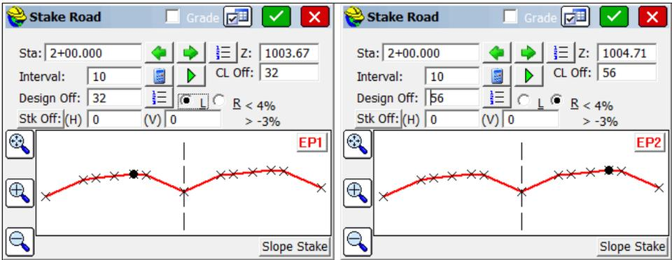
Shown below is a staking of a Horizontal Offset of 4 from the outside right shoulder, extending the shoulder slope to the right on station 210.
