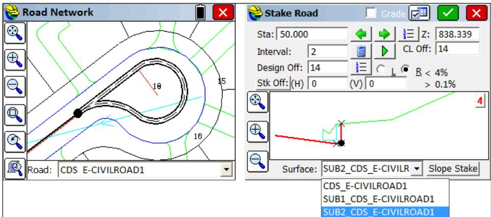
The cul-de-sac "centerline" is the outside edge-of-pavement facing the curb, and by clicking "From List" opposite Station, is seen to be just over 200 in total length in the screen below left. Staking out station 50 would be approximately 1/4 of the distance around the cul-de-sac.
