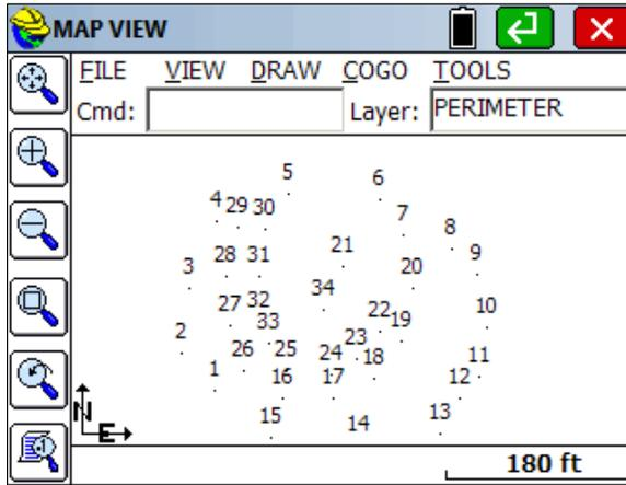
So, using the settings above in the Volume routine, you would verify your two point ranges, then click OK. For example, the “Original” surface point range would be set as follows using the “Define” button for “Original” prior to clicking OK.
