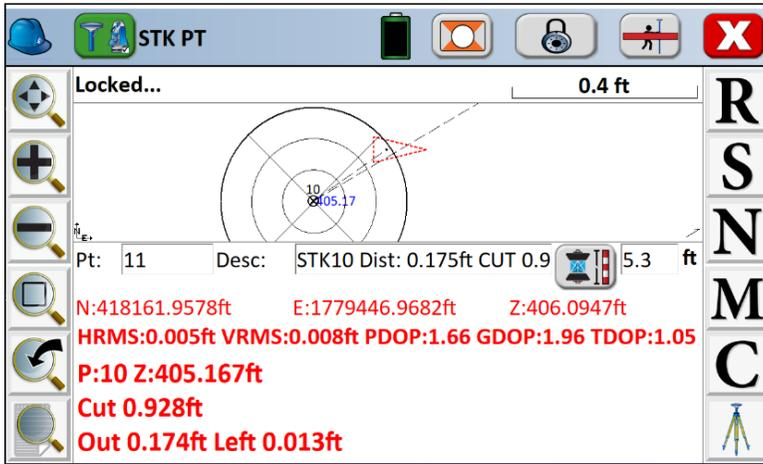
*Shown in the image above, the robotic total station is the active instrument, but it is in a locked state (the E.D.M. is not firing). Since no position is available from the active instrument, and backup tracking is enabled, SurvCE is displaying the backup stakeout directions from the GPS position in red.*
