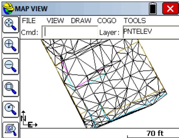
The 3DFaces are placed on a layer (TRI\_FACE by default), and that layer can be turned off and removed from view. If you choose E for Erase, you can pick the 3D Face entities and erase them on command. There is no particular value to seeing the 3D Faces, so it is not recommended that they be drawn. The main value is to capture the TIN (triangulation) file for use in Elevation Difference.
