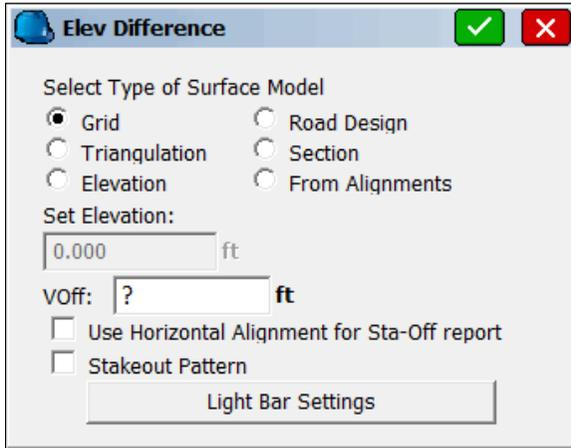
For example, grading a site that had 4 subgrades with a modeled top surface, you need to grade to the lowest subgrade surface with a vertical offset of  $(0.12+0.15+0.33+0.25)$ . Quickly obtain the value by entering '?' in the Vertical Offset field within the Elevation Difference dialog, as shown above.
