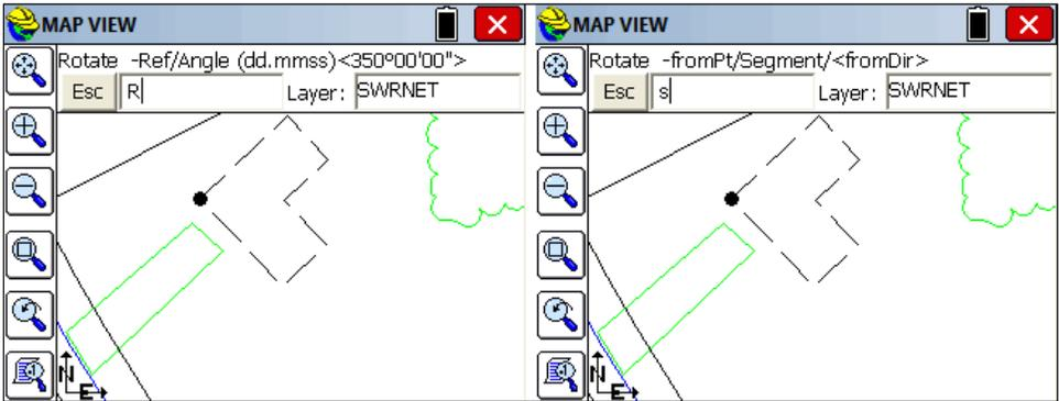
Select the pivot point first. If you want to make it parallel to an existing line, choose R then S for Segment, then pick the segment on the figure you wish to reference first. Then after that, the next pick, also by S for Segment, will be for the property line (e.g. the line to the north) you wish to match.
