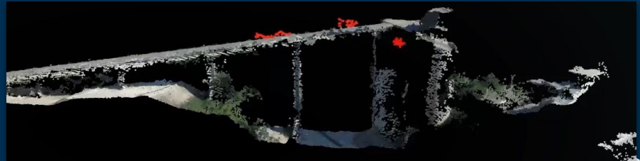
REMOVE EXTRANEOUS POINTS FROM THE POINT CLOUD IN PIX4Dmapper
