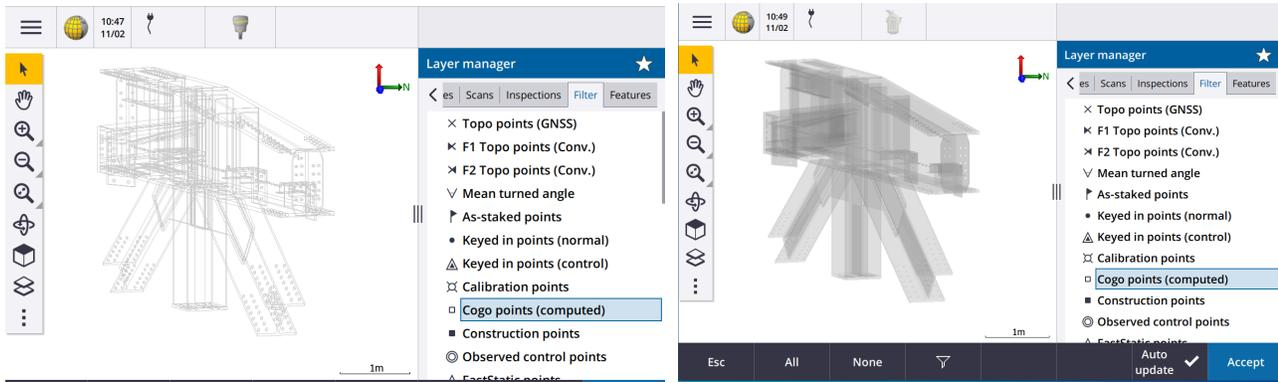
Trimble Access also includes a limit box functionality to section out specific areas of the model. This is very handy if only a specific part of the model is needed:
