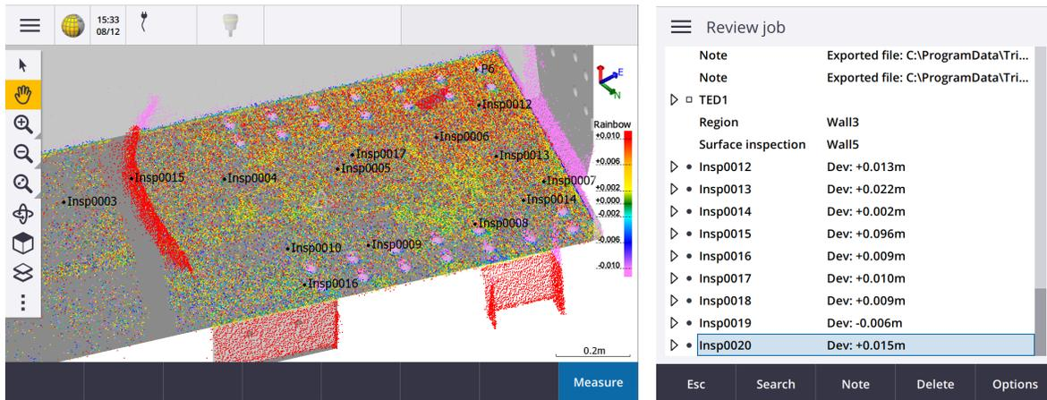
The “Inspection to surface” can also be done with prism measurements through the function “Measure Surface”. In this case, when taking a measurement to the prism, the system will calculate the perpendicular deviation value between the measurement and the underlying 3D model surface.
