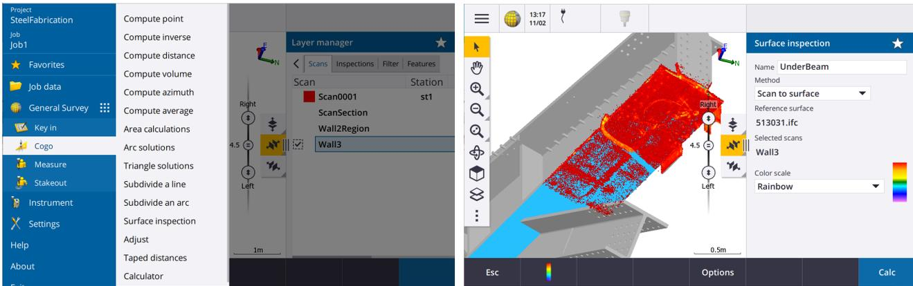
When the calculation is complete, an instant deviation value between the as-built object and the design data can be presented by simply selecting the specific point of interest. By pressing “Store” a snapshot of the screen is taken and the selected deviation points are stored. The inspection data is stored in a separate tab under the layer manager, which makes it easy to select and check individual deviations.
