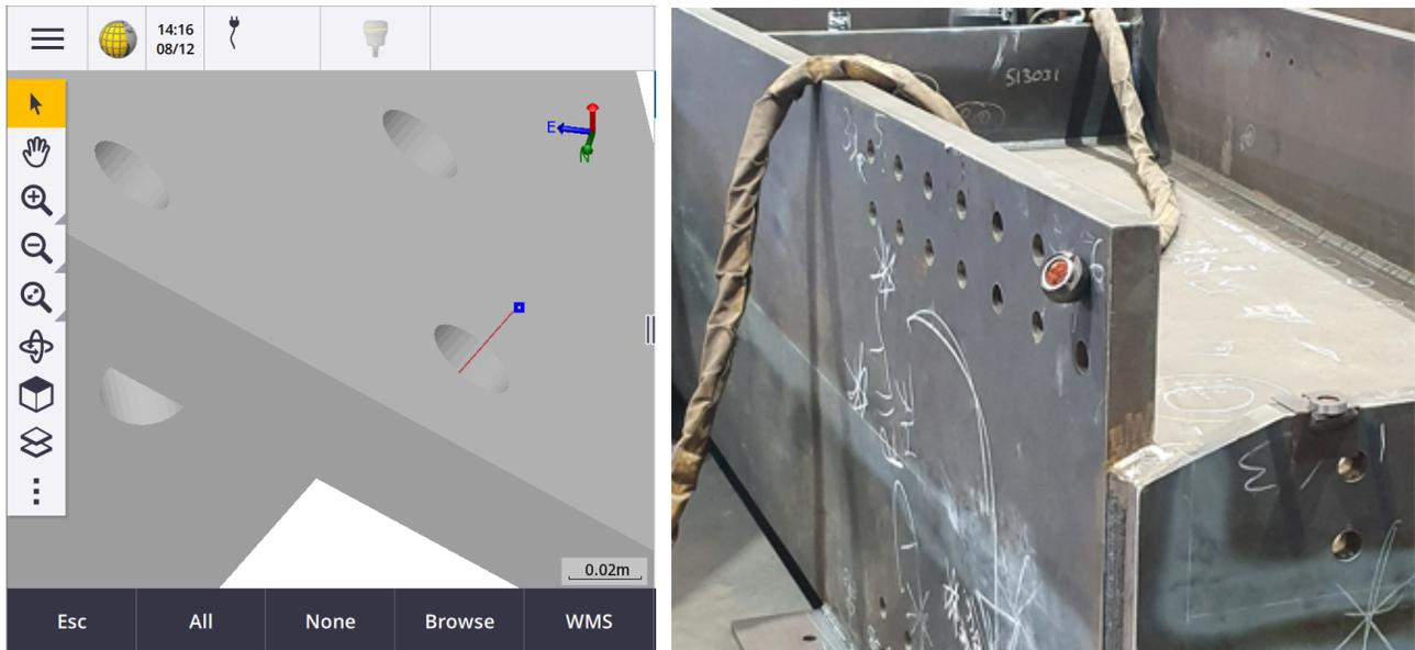
As soon as an observation is taken, the data is stored in Trimble Access. If the selected control points have been pre calculated and the user observes these, the deviation between the calculated and the observed point is automatically stored in the Trimble Access database and this can be exported afterwards as a report.
