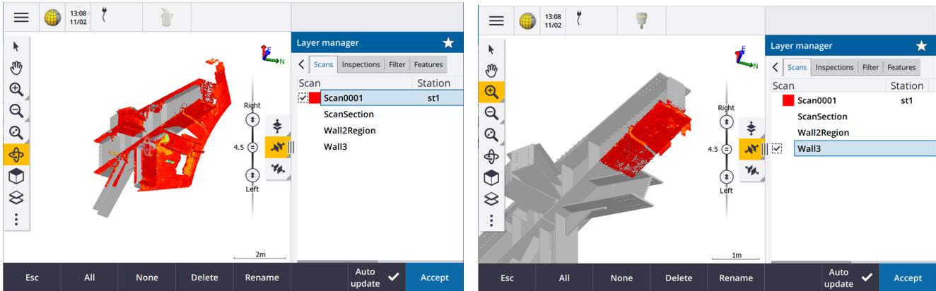
The scan-to-model comparison is a functionality that can be found under the COGO menu. Users can choose “Surface Inspection” and then pick the surface they want to inspect; that can be an individual surface or a whole object. Next, the inspection should be given a name and the map configuration should be chosen (this can be individually configured based on the needs of the inspection, required tolerances, colours of tolerances, etc.).
