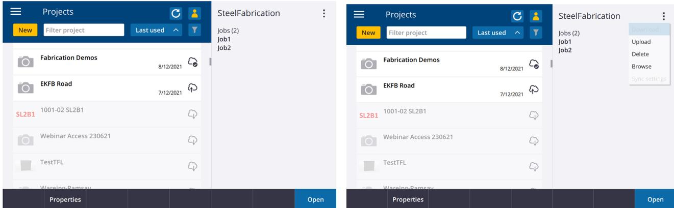
By pressing the download button users can select the specific file(s) they want to work with. The file will be downloaded to Trimble Access internally and users can manage which one to work with through the Layer Manager. Multiple model files can be used, if required - there is no restriction to only display one model at the time (e.g. 3D model and annotations, set out points, etc.).
