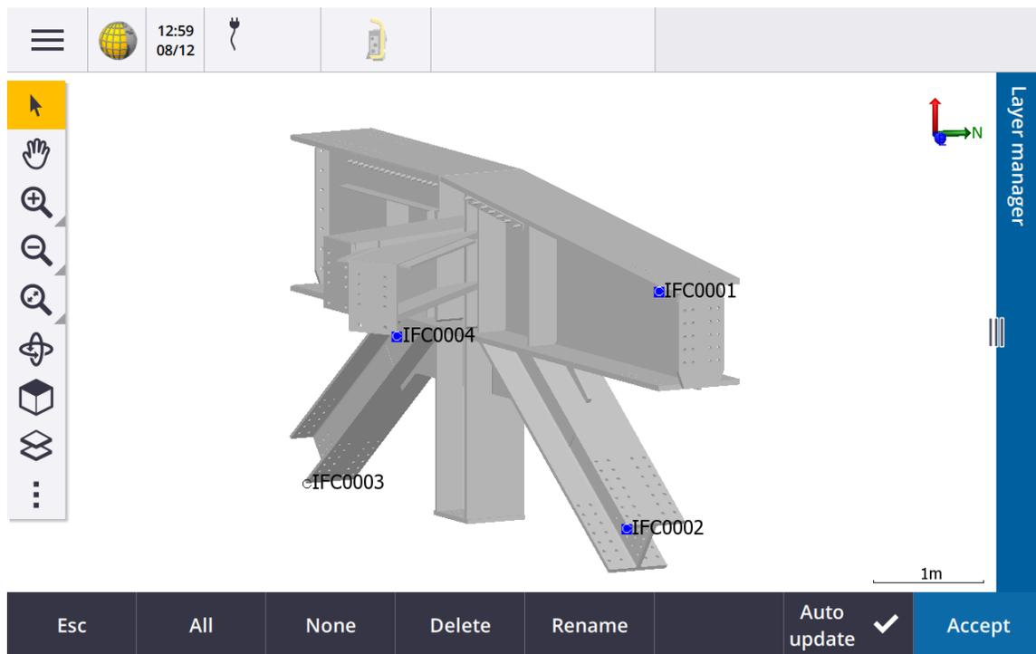
The registration process is completed when 3 points have been captured. However, users can choose to add more points in order to build redundancy.
