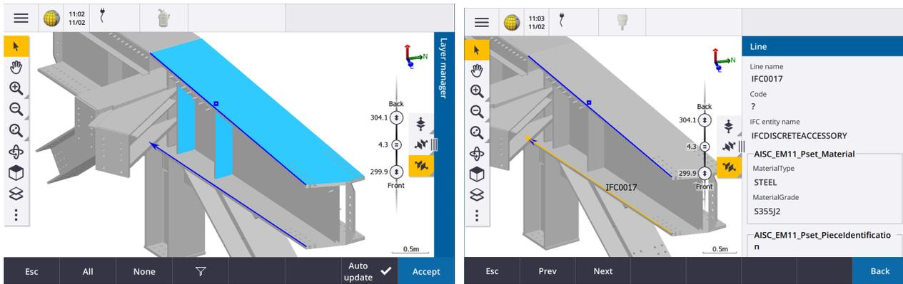
In terms of the Object oriented Set-Up process, the user will need to pick 3 points and then observe each of these in order to get the set-up done. Users can either pick 3 points and store them and then select these as they observe. However, it's easy enough to pick a point in the model, then turn the Total Station to this point on the real model and observe. This needs to be done minimum of 3 times to get a solution.
