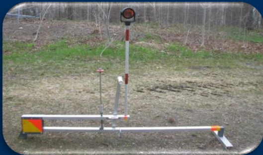
Survey rail coordinates with rail shoe and track bar
